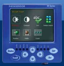
The setup mode allows the configuration of the image quality parameters, selects and re-sizes the control area and chooses the processing tool to use.
