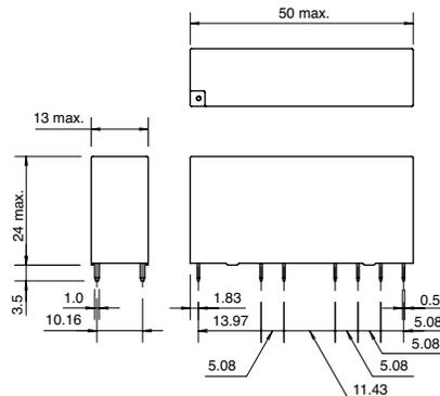
PC Board Terminal type Mounting Hole Layout (Bottom View)
