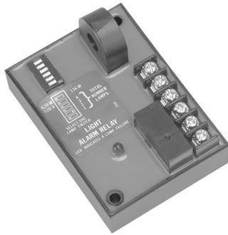
The SCR series is a universal lamp alarm relay designed to sense the failure of flashing or steady incandescent beacon lamps or steady side lights. The toroidal current sensor provides isolation and allows monitoring of more than one line at a time. The SCR Series energizes when one or more lamps fail. It will monitor the operation of one to four side lights and up to four beacon lamps.
