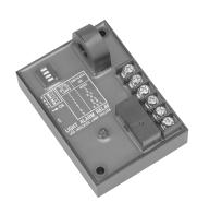
The SCR490D Series is used to provide remote monitoring of steady burning incandescent marker and obstruction lighting. Four onboard switches allow operator programming for lighting systems with two through nine lamps on a single AC circuit. The SCR490D uses a toroidal sensor and electronic circuitry to sense the failure of one or more lamps.
