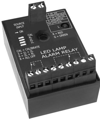
The SCR series is a universal lamp alarm relay designed to sense the failure of flashing or steady LED beacon lamps or obstruction lamps. The SCR Series energizes when one or more lamps fail. It will monitor the operation of one to eight beacon or obstruction lamps. All monitored lamps must be the same wattage and voltage. When connected to a site monitoring system, it provides the remote lamp monitoring protection required by the FAA-AC No: 150/5345-43E.
