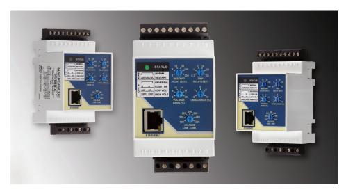
Troubleshooting is easy with full fault indication on the front face. Dials allow adjustment of undervoltage trip point, trip delay, restart delay, unbalance trip point and selection of line-to-line system voltage.
