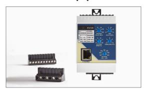
Compact 60 mm wide enclosure mounts on DINrail or can be panel mounted with two screws inserted through clips that extend from the back of the enclosure. Pluggable terminal blocks on both the inlet and output side enable easy installation and replacement without removing any wires.
