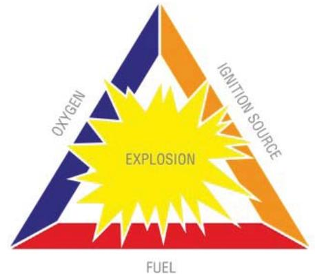
**Note:** both the flammable substance and the oxygen must be present in the correct mixture for the explosion to happen.
