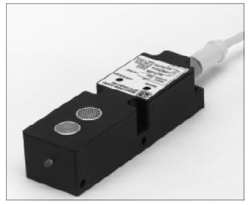
also features a quick disconnect receptacle. The housing is constructed of plastic valox and has standard 30mm X 60mm limit switch mounting dimensions, as well as side holes for mounting the sensor on its side. The output consists of two solid state relays N.O. N.C., and can switch 2 - 130VAC or VDC up to 100mA DC or 50mA AC continuous. The relay outputs are short circuit protected and isolated up to 1500 volts rms.
