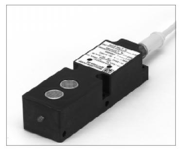
place, depending on how much reflected signal is coming back from the target. The frequency of operation is 38.5kHz. There are two ranges available in this model 2" to 40" or 5" to 80". It also features a quick disconnect receptacle. The housing is constructed of plastic valox and has standard 30mm X 60mm limit switch mounting dimensions as well as side holes for mounting the sensor on its side.
