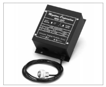
analog outputs are supplied. The RPS-300 sensor operates at a frequency of 222kHz for the 14" and 36" ranges and 150kHz for the 72" range. This sensor has a narrow sensing beam. Sensing ranges available for the RPS-300 include 4" to 14", 5" to 36", and 8" to 72". Mounting flanges, LED indicator, ranging potentiometer and 6-ft. transducer cable are included. Optional cable lengths are available.
