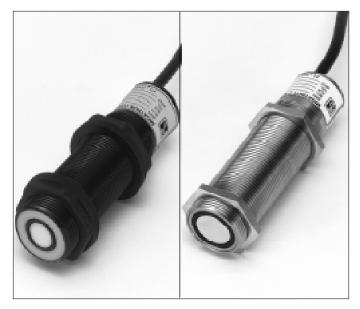
set up purposes an LED indicator is provided. When not detecting the LED will illuminate green and when detecting the LED will illuminate red. The outputs consist of two solid state relays N.O. N.C. which can switch 2-130VAC or VDC up to 100mA DC or 50mA AC continuous. The relay outputs are short circuit protected and isolated up to 1500 volts rms. A standard 6' cable is provided. An optional quick disconnect plug is available.
