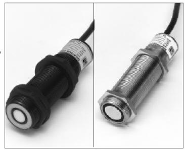
the target. The frequency of operation for the RPS-401A is 212kHz for the 4" to 40" and 150kHz for the 8" to 80". The RPS-426A has a 8" to 80" range and operates at a frequency of 150kHz. The RPS-401A barrel is constructed of plastic valox, and the RPS-426A is Stainless Steel. The barrel measures 30mm x 100mm. A standard 6' cable is provided. An optional quick disconnect plug is available.
