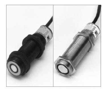
The LED indicator illuminates when the ultrasonic wave from the sensor is reflected back to the sensor within the preset range. These sensors provide precise proximity or level sensing regardless of color, density, or transparency. They are equally effective on liquid, metal, plastic, and glass targets.
