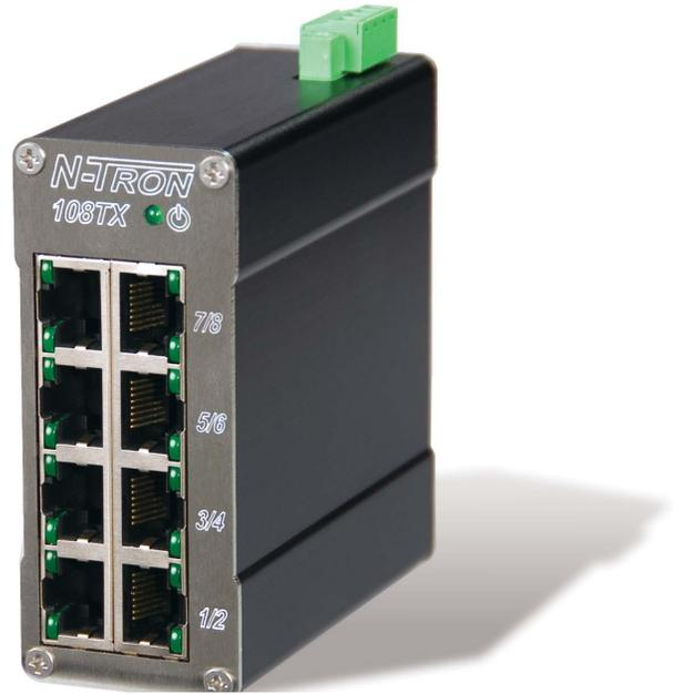
The 108TX supports up to 2,000 MAC addresses, enabling these products to support extremely sophisticated and complex network architectures.
