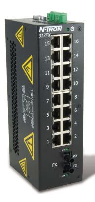
The 317FX-N simplifies plant wiring by eliminating the need to bring data acquisition and control connections back to a climate controlled environment. The switch has extended operating specifications to meet the harsh needs of the industrial environment, including extended temperature rating, extended shock and vibration specs, redundant power inputs, and a high MTBF (greater than 2M hours).
