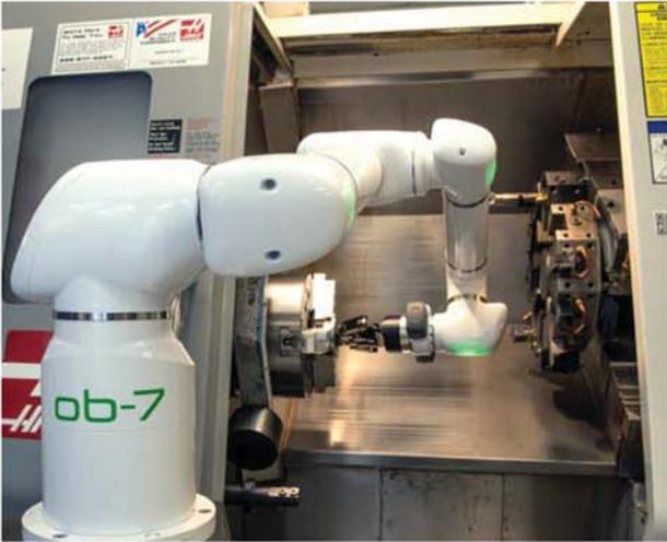
**Machine Shop Loading & Unloading**
