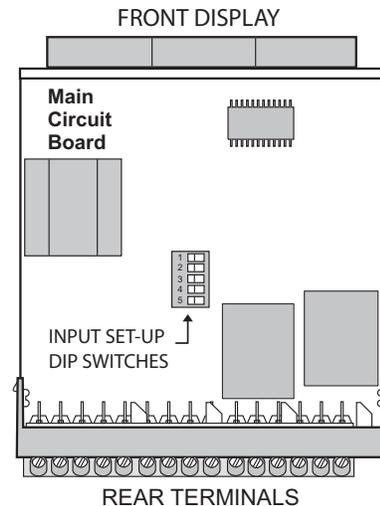
*Note 1: When the DIP switch is in the SNK position (OFF), the signal input is configured as active low. When the switch is in the SRC position (ON), the signal input is configured as active high.*
