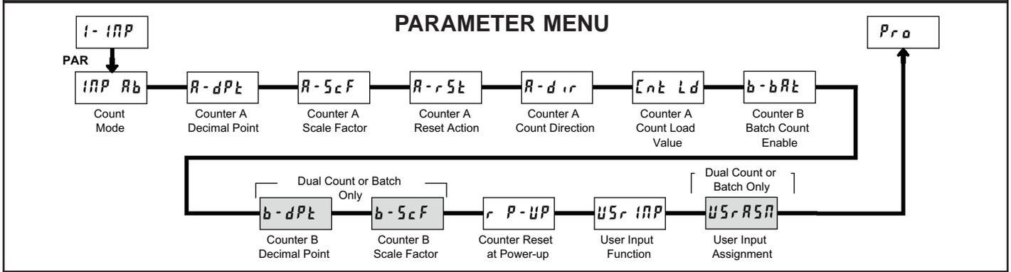
Shaded area selections only apply when Counter B is enabled (Dual Count mode or batch counter).
