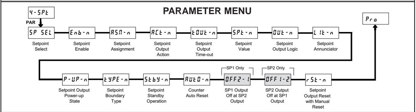
Some Setpoint parameters will not appear depending on the Setpoint Assignment and Setpoint Output Action selected. The Setpoint Parameter Availability chart below illustrates this.
