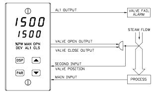
The motorized valve positioner controls the position of a valve directly, by use of "open" and "close" control outputs. The slidewire feedback signals of the valve may optionally be connected to the controller. Alternatively, the controller may be configured for linear input valve control using the 4 to 20 mA DC output.
