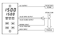
The motorized valve positioner controls the position of a valve directly, by use of "open" and "close" control outputs. The slidewire feedback signals of the valve may optionally be connected to the controller. Alternatively, the controller may be configured for linear input valve control using the 4 to 20 mA DC output.
