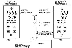
Similar to internal cascade control, external cascade control differs by the employment of two controllers, one of which is equipped with a second analog input configured as a remote setpoint. A PCU controls the secondary loop, while a TCU controls the primary loop. - -
