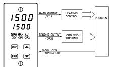
The TCU has dual outputs for providing heating and cooling to those processes that require them. Many extruder applications require both heating and cooling to maintain accurate extruder barrel and die temperatures. The TCU is easily configured for these applications.
