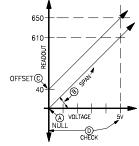
Example 3 (Negative Slope): A liquid level sensor puts out 1 V when a storage tank is full and 11 V when the tank is empty. The APLPV is to readout 100.0 when the tank is full and zero when the tank is empty.
