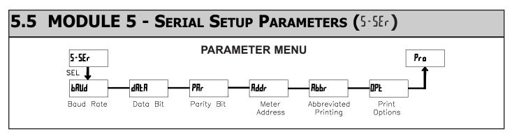
The Serial Setup Parameters are only active when the optional RS232 or RS485 serial communications module is installed in the meter. Refer to the CUB5COM bulletin for complete details on CUB5 serial communications.
