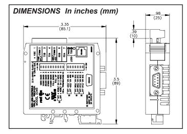
The unit is equipped with a universal mounting foot for attachment to standard DIN style mounting rails, including top hat profile rail according to EN 50 022 - 35x7.5 and 35x15, and G profile rail according to EN 50 035 - G32.
