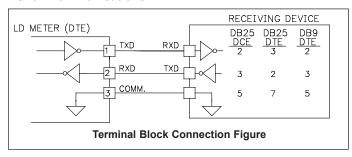
RS232 is intended to allow two devices to communicate over distances up to 50 feet. Data Terminal Equipment (DTE) transmits data on the Transmitted Data (TXD) line and receives data on the Received Data (RXD) line. Data Computer Equipment (DCE) receives data on the TXD line and transmits data on the RXD line. The LD emulates a DTE. If the other device connected to the meter also emulates a DTE, the TXD and RXD lines must be interchanged for
