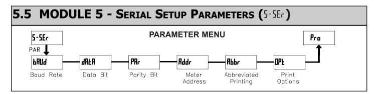
Module 5 is the programming module for the Serial Communications Parameters. These parameters are used to match the serial settings of the LD with those of the host computer or other serial device.
