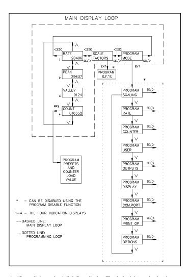
significant digits on the 6-digit Rate display. The desired time units that the rate is to be displayed, can also be programmed as per Second (xI), per Minute (x60), or per Hour (x3600).
