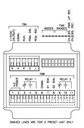
(The input connections are the same for 1 or 2 preset timers.)
