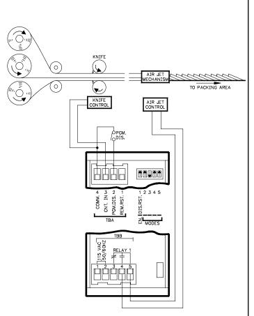
The preset number and output time duration are locked from further entry when the key switch connects the Program Disable ("PGM. DIS.") terminal to the "COMM." of the LYNX Contact Counter.
