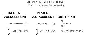
Note: In the figures above, the text shown in parenthesis is printed on the circuit board to help with proper jumper positioning.
