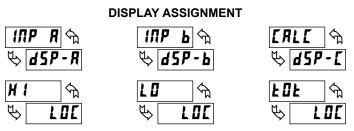
There are six meter values that can be individually programmed for one of the main displays (A,B,C or \_), or programmed to be viewable in Quick Programming mode (rEd), or programmed to be locked out from display (LOC) (see the following table). If two or more values are assigned to the same display the last value assigned will be the one that is displayed.
