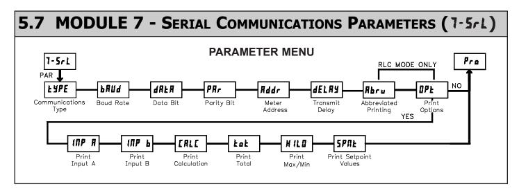
Module 7 is the programming module for the Serial Communications Parameters. These parameters are used to match the serial settings of the PAXDP with those of the host computer or other serial device, such as a terminal or printer. This programming module can only be accessed if an RS232 or RS485 Serial Communications card is installed.
