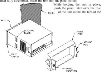
panel latch engage in the slots on the case. The panel latch should be engaged in the farthest forward slot possible. To achieve a proper seal, tighten the latch screws evenly until the unit is snug in the panel (Torque to approximately 7 inlbs [79N-cm]). Do not over-tighten the screws.
