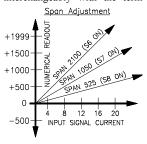
readout for a given input signal current change. The input summing resistor values are weighted in a binary progression, so they can be switched in combinations to give 32 discrete steps of span. The fine adjust control brackets these coarse steps and can be adjusted to the exact span needed.
