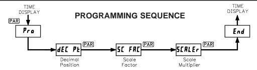
The Process Time Indicator has three programmable parameters which are entered in the sequence shown above, using the front panel push buttons.
