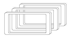
The Gemini Series panel adapter kit permits the mounting of the Gemini unit to an existing 68 mm x 138 mm DIN standard panel cut-out. The kit consists of two metal adapter plates coated with a durable flat black polyurethane finish, and a neoprene gasket, which provides a sealed front panel that meets NEMA 4/IP65 specifications when properly installed.
