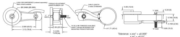
MOUNTING: Pivot Shaft can be mounted from either side of the housing and is field reversible.
