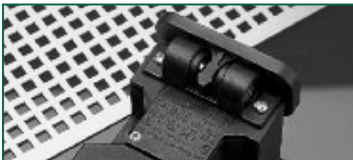
AZ15/16-2053 with ball catch Holding force up to 22 pounds
