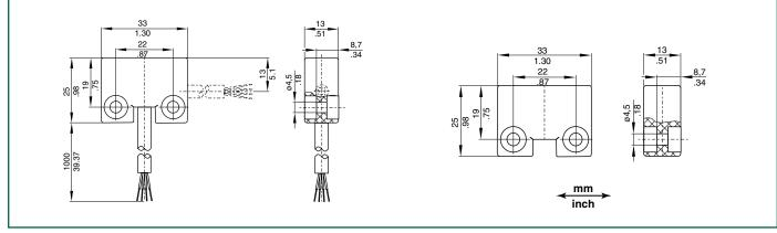
Note: BNS250 reed switch assemblies should be mounted at least 50mm (2") apart.
