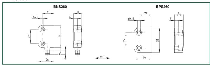
Note: BNS260 reed switch assemblies should be mounted at least 50mm (2") apart.
