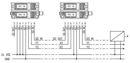
Y1 and Y2 = Safety outputs SD-IN Gateway Field bus
