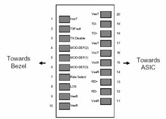
**SFP Transceiver Electric Pad Layout**
