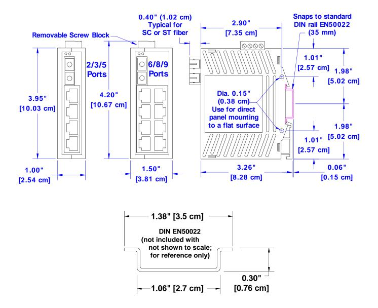
Figure 3a – SL Enclosure Mechanical Dimensions
