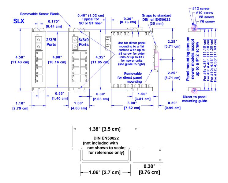
Figure 3b – SLX Enclosure Mechanical Dimensions
