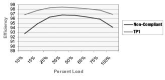
75 kVA Transformer Efficiency
