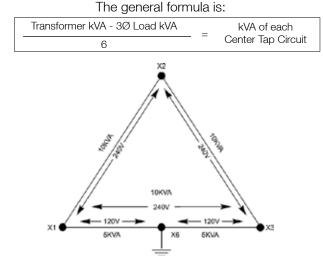
Note: All 480 delta to 240 delta transformers stocked by SolaHD are equipped with a center tap.
