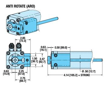
NOTE: When ARO is used together with FFG stroke is reduced by 0.45" [11.4 mm]
