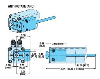
NOTE: When ARO is used together with FFG stroke is reduced by 0.51" [13.0 mm]
