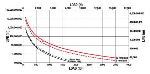
NOTE: The L<sub>10</sub> expected life of a ball screw linear actuator is expressed as the linear travel distance that 90% of properly maintained ball screws manufactured are expected to meet or exceed. This is not a guarantee and this graph should be used for estimation purposes only.
