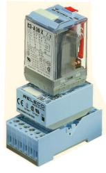
The modules **CT2** and **CT3** are electronic timers that are designed to be inserted beween a standard plug-in relay and its socket, enabling the relay to be operated as a timer relay.
