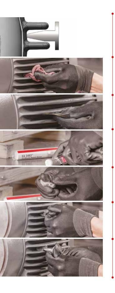
Always verify the sensor receiver mount is the correct size for your motor. It must be thin enough to fit between the cooling fins in a preferred location according to the installation instructions found on page 2 of this manual. The sensor receiver must be long enough to make contact with the motor frame and extend beyond the cooling fins. Loctite™ 3463 putty will be used to fill the gaps between the cooling fins and the sensor receiver mount.
