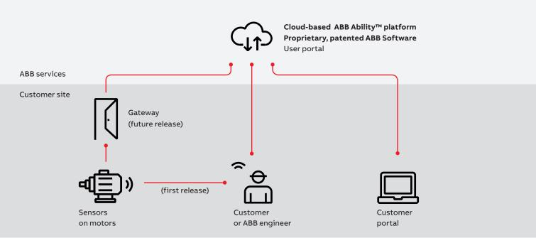
ABB's condition monitoring solution for LV motors. The ABB Ability™ Smart Sensor transmits data via a smartphone (first release) or gateway to a secure cloud service. Algorithms in the cloud analyze the data and convert it into meaningful information, which is then sent to the user's smartphone and customer portal.
