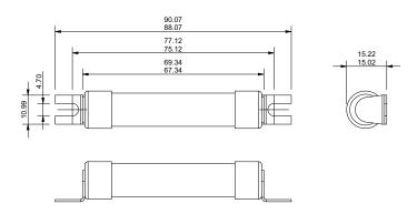
Cylindrical with 10mm Fixings PV-(amp rating)A14LF10F
