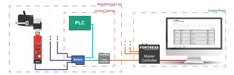
Local controller provides robustness and line-side communication
